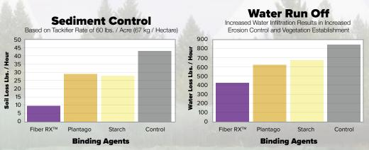
"Test results completed at the Rainfall Simulation Facility at Utah Water Research Laboratory, Utah State University using a 2,000 lb / Acre (2,250 kg / hectare) Rate Wood Fiber slumy mix with 60 lbs / Acre (67 kg / hectare named Tackifier. Products applied on 3:1 slope, allowed to dry, and rained on at 3 in. (7.6 cm) / hour rate, results recorded at 30 minutes.
